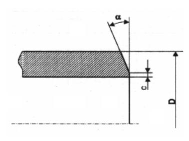
Figure 1 — Tube end bevel
